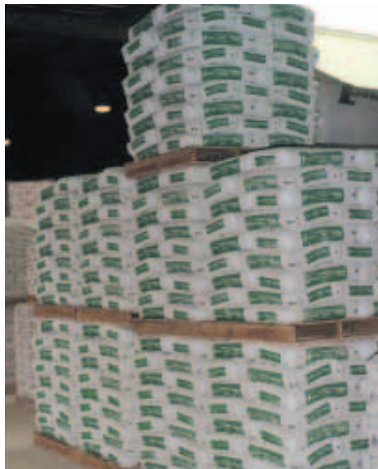
Top, the Lock n' Pop adhesive is sprayed on Lafarge cement bags, which can then be piled high on pallets (bottom) without stretch wrap.
